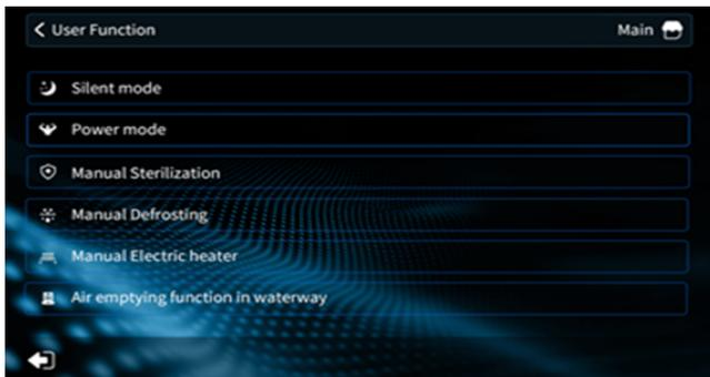
**Silent mode** Can be touched anytime to activate or deactivate silent mode. In quiet mode the compressor /fan motor operates at low frequency and the capacity of the unit is reduced.
