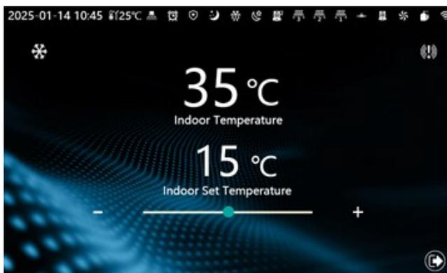
Dual Heating zones and Indoor Circulation Pump function can only be selected to enable one of them. P150 is used to enable/disable functions. (1-Runs on power-up/ 2-Controlled via linkage switch/ 3-Controlled by room temperature). Once installed, the wired controller with built-in temperature sensor will automatically detect the indoor ambient temperature and display it in the top status bar of the wired controller.
